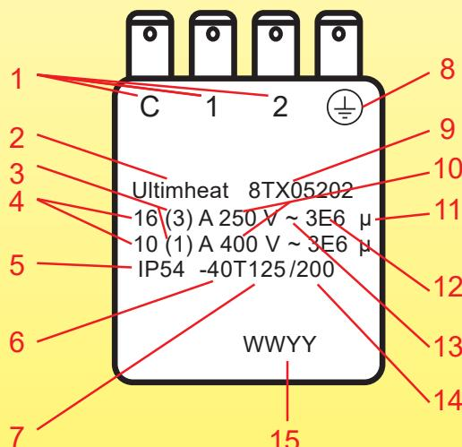
1: Identification of terminals that are suitable for the connection of external conductors, and if they are suitable for line or neutral conductors, or both.
