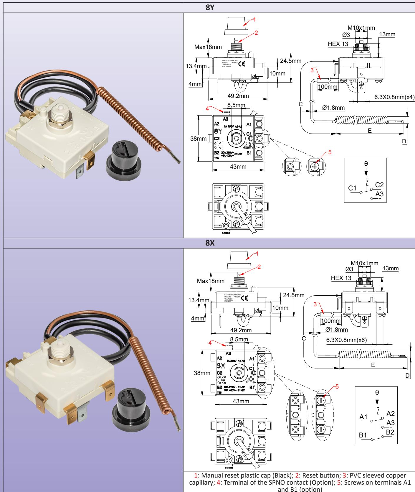
1: Manual reset plastic cap (Black); 2: Reset button; 3: PVC sleeved copper capillary; 4: Terminal of the SPNO contact (Option); 5: Screws on terminals A1 and B1 (option)
