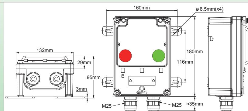
3 x 16A (AC1), 250V, terminal block with 5 terminals 2.5mm<sup>2</sup> screws and 5 screw terminals 6mm<sup>2</sup>. Red indicator light for power supply and output green light (250V), transparent window.
