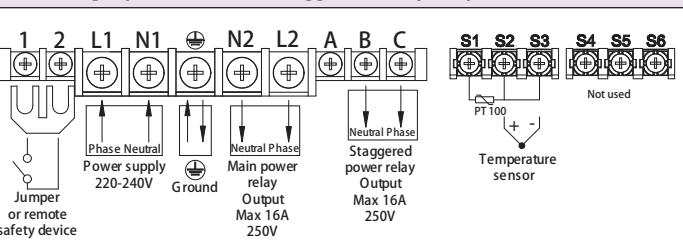
3 pole circuits, 2 staggered relay outputs 3x16A 250V
