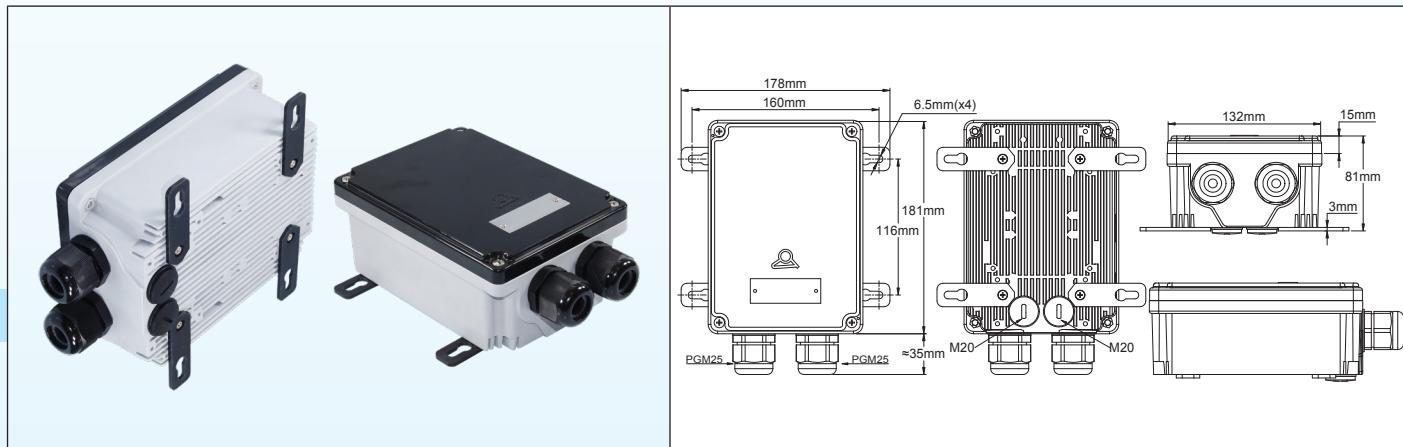
These sealed aluminum boxes are RAL 7015 epoxy painted. They have the same dimensions than the plastic control boxes, and use flat lids. They use the same wall mounting tabs than plastic models. They have been designed for mounting of single or three phase solid state relays of which the cooling is carried by the fins on the rear face.
