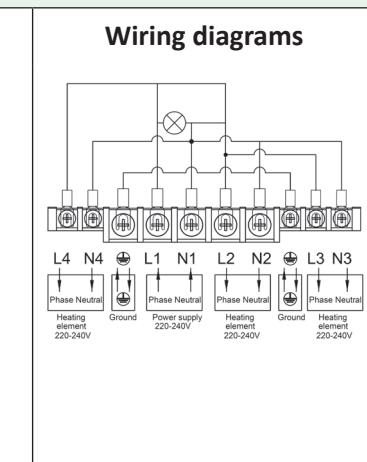
**Wiring:** power supply Neutral + Phase + Ground on a 6mm<sup>2</sup> terminal block, and outlets to 3 heating circuit outlets 1.5 or 2.5mm<sup>2</sup>.
