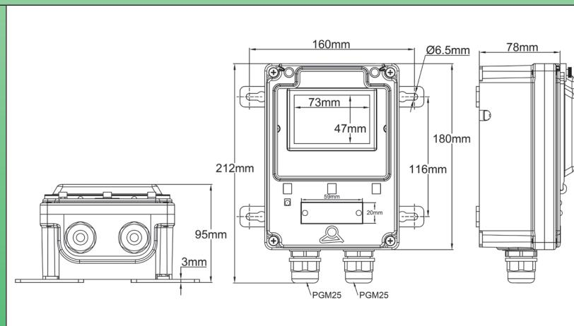
Allows mounting of a circuit breaker type Merlin Gerin Multi 9 (UL, CSA, IEC) and equivalent European ranges Vigi C60 or C60 (72mm maximum width = four 18mm modules), or electronic controllers described in this catalogue
