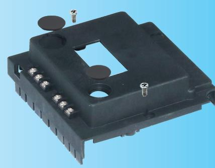
Extended mounting board, in PA66, with 71 x 29mm rectangular hole for 78 x 35mm controller
