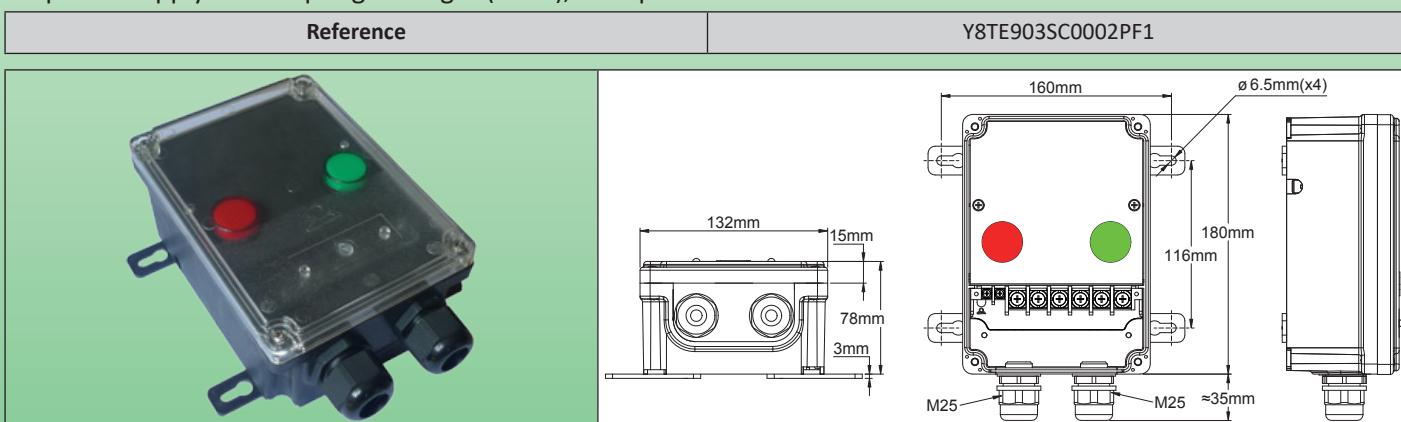
3 x 25A (AC1), 250V, terminal block with 2 terminals 2.5mm<sup>2</sup> screws and 6 screw terminals 10mm<sup>2</sup>. Red indicator light for power supply and output green light (250V), transparent lid.
