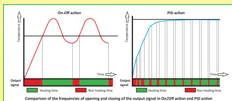
If the PID action can improve the control in a number of configurations, the drawback is that the output signal will cycle very quickly, which reduces the power relay life very extensively and requires in most cases to use solid state relays.
