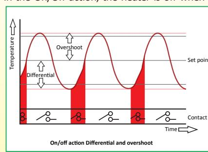
**Adjustable differential:** A low differential is often associated with control accuracy. However, a too low differential will cause heating short cycles and premature contact wear if a power relay is used, or a quick degradation of the compressor if the system is used to control a refrigerator. The electronic controllers in this catalog have an adjustable differential to optimize this operation.
