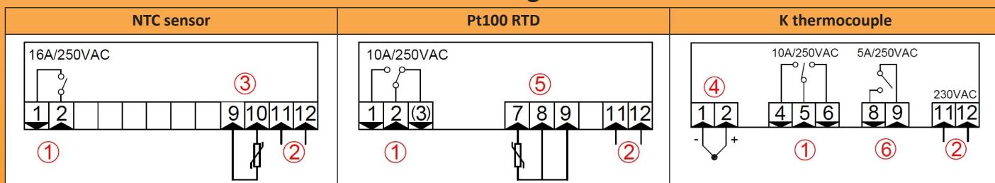
1: Relay output; 2: 230V AC power supply; 3: NTC sensor; 4: K thermocouple sensor; 5: Pt100 sensor; 6: Alarm relay output.
